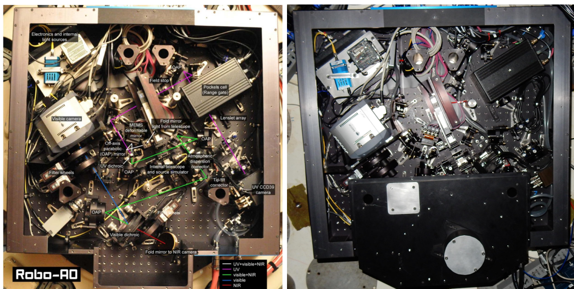
Figure 1. Images of the Robo-AO Cassegrain instrument at Palomar ( left ) and at Kitt Peak ( right ). The light from the telescope enters the instrument with a fold mirror and onto an OAP which images the pupil onto the MEMS deformable mirror (white line path in the Palomar image on the left). Then a UV dichroic splits the UV light (magenta), which passes through a condenser lens, onto an OAP, into the Pockels cell, through a lenslet array, and onto the Shack-Hartmann wavefront sensor while the visible and infrared light (green) passes through a second OAP relay, which includes the atmospheric dispersion corrector (ADC) and tip-tilt corrector (currently not in use, see text in §2). A visible dichroic then sends the visible light (blue) to the visible CCD camera and infrared light (red) to the soon-to-be deployed infrared camera. The large black platform at the bottom of the Kitt Peak image is the mount for the infrared camera.
