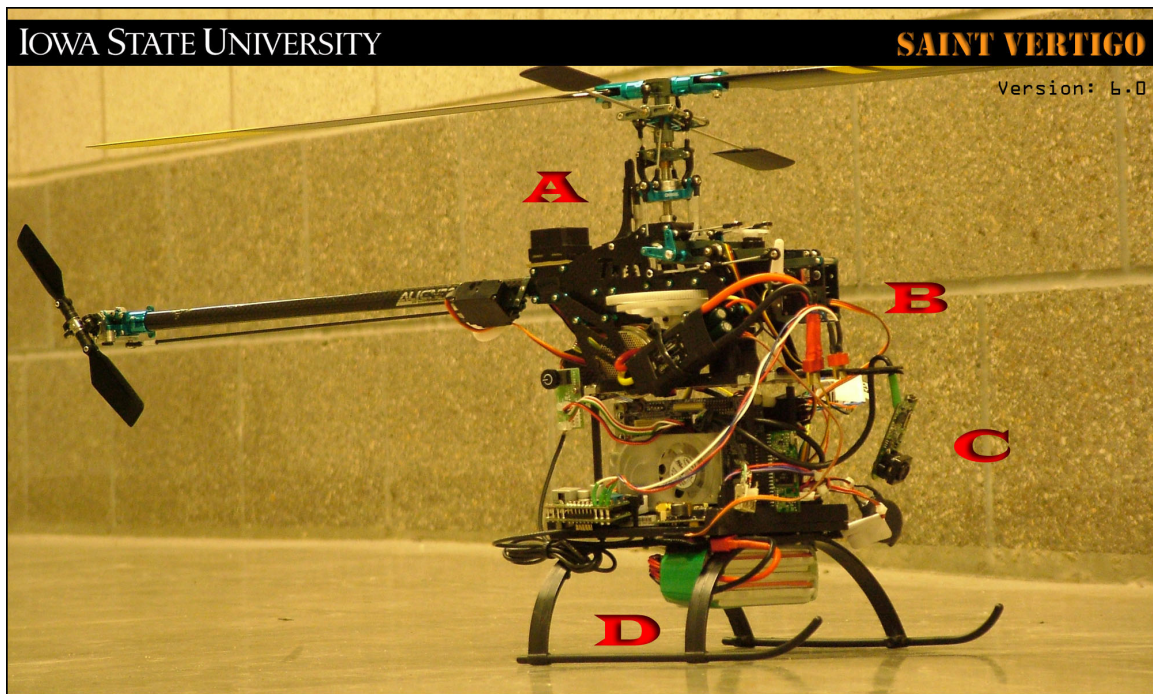
Figure 14. The Saint Vertigo, Iowa State's MAV helicopter, consists of four steel reinforced carbon fiber decks. The A-Deck contains collective pitch rotor head mechanics with mechanical mixing. B-Deck comprises the fuselage which houses the power-plant and controller, transmission, actuators for flight surfaces, rate gyroscope, compass, and the tail rotor. C-Deck contains the brains of Saint Vertigo; an autopilot computer, a navigation computer, an inertial measurement unit, a 2.4 Ghz manual override with double redundancy for fault tolerance, a 900 MHz wireless modem, a 802.11 wireless network device, a 2 megapixel digital video camera, and a collection of sensors including an ultrasonic altimeter, a barometric altimeter, a pitot tube, and a GPS module. D-Deck is the undercarriage designed to act as a shock absorber. This deck also provides a wired ethernet port, a USB port and a VGA port for programming purposes. D-Deck also features hardpoints for attaching the fuel cells, with options available to carry one at the expense of flight time, or two at the expense of maneuverability, depending on the mission requirements.
