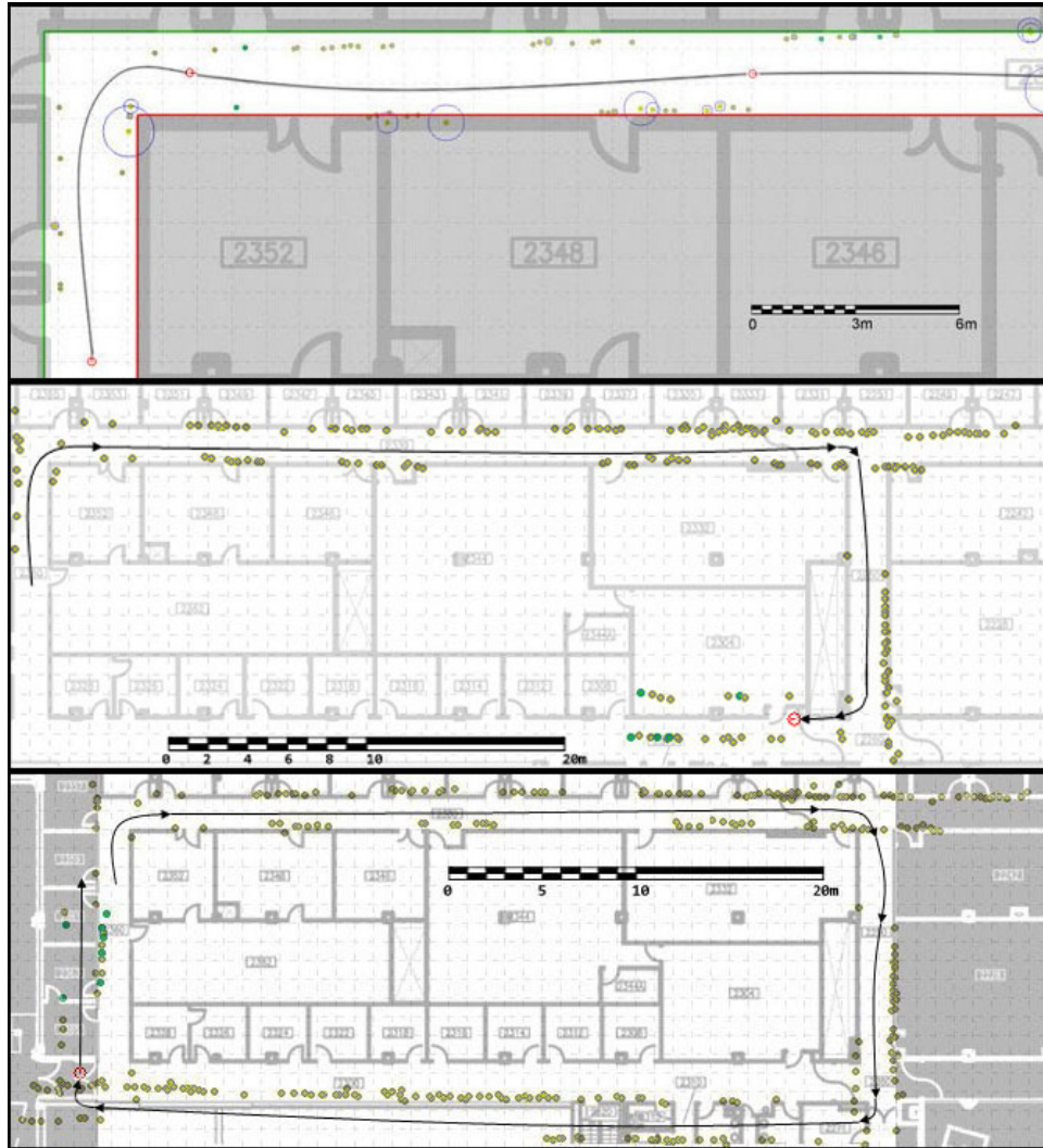
Figure 13. After completing a single 104 meter loop the MAV returns to the starting point. The proposed ranging and SLAM algorithm closes the loop with less than 2 meters of error. It should be stressed that building floor plan was superimposed on this image after the mission is complete to provide reference data for the ground truth to demonstrate the performance and accuracy of our method. It is not provided to the MAV a-priori. The error is introduced in the third leg of the hallway which consists of flat white walls.
