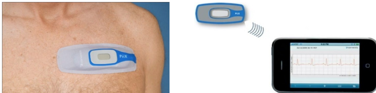
Figure 5. Another example of a wireless sensor technology for real-time ECG monitoring. Picture Credit: NASA.
