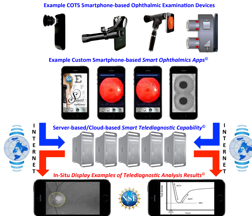
Figure 1. Schematic overview (extracted from [5, 6]) of Smart Ophthalmics ® : a smart service platform in ophthalmology.
