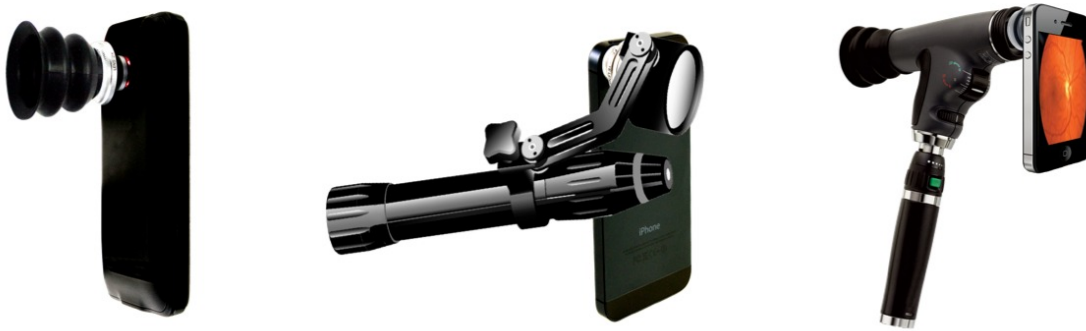
Figure 2. Examples of smartphone-based ophthalmic examination devices: ophthalmic microscope (left); ophthalmic slitlamp by Eidolon (middle); and ophthalmoscope/funduscope by Welch Allyn (right).
