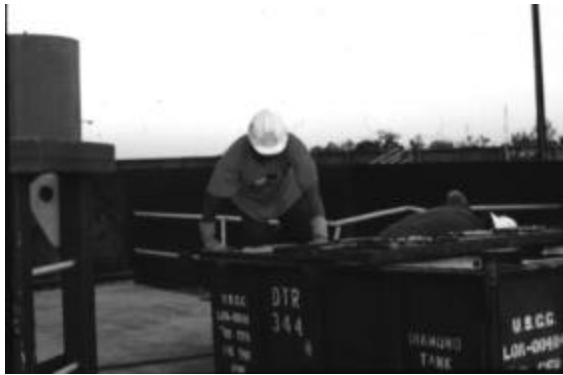
Figure 3.2. Contract laborer cleans mud tank
