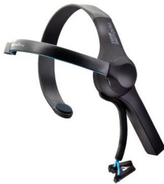
(a) NeuroSky MindWave Mobile single-channel headset [11]
