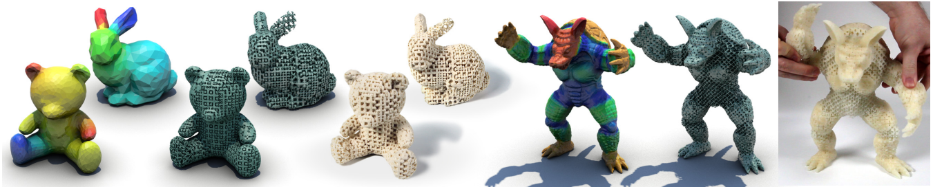
Figure 1: Given a virtual object with specified elasticity material parameters (blue=soft, red=stiff), our method computes an assemblage of small-scale structures that approximates the desired elastic behavior and requires only a single material for fabrication.
