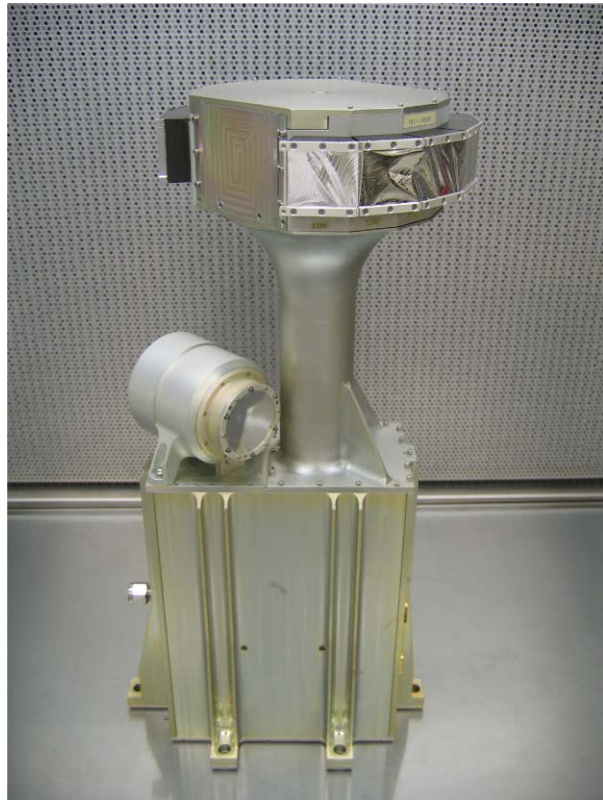
Fig. 3 Photograph of LET ( top center ), HET ( center left ) and SEP Central ( enclosure at bottom ). Overall height is approximately 43.4 cm. The bottom of SEP Central is elevated \frac{3}{4} " (1.9 cm) above the spacecraft deck due to thermal isolators
