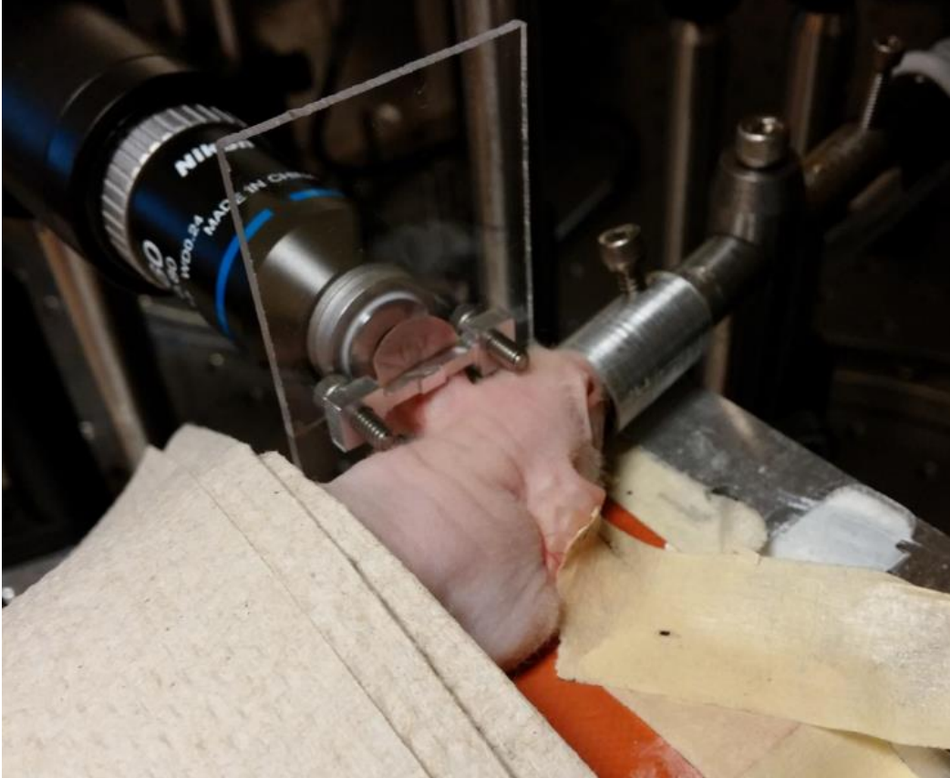
Supplementary Figure 4. A photo of the set-up used to measure the speckle correlation time after blocking the blood flow in the mouse ear. A metal bar pressed the ear against a stiff acrylic wall to block its blood flow.
