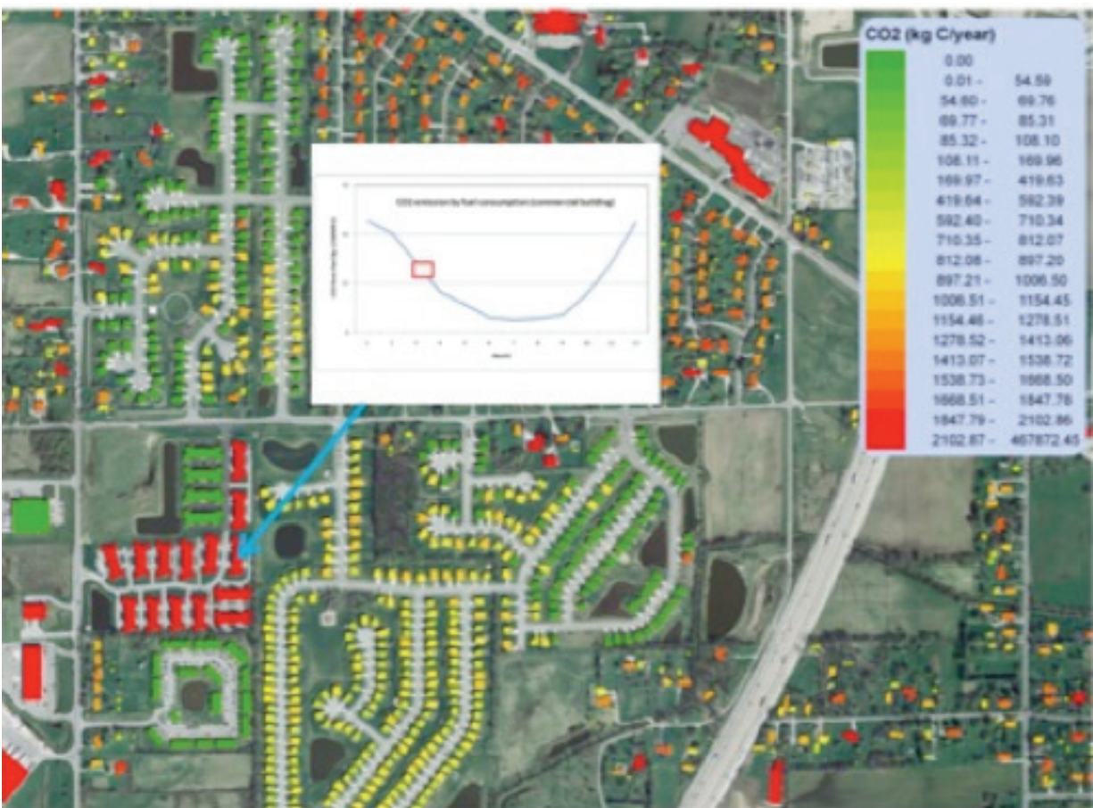
Figure G-2. An example of the bottom-up, building resolution, emissions estimate from the Hestia project.
