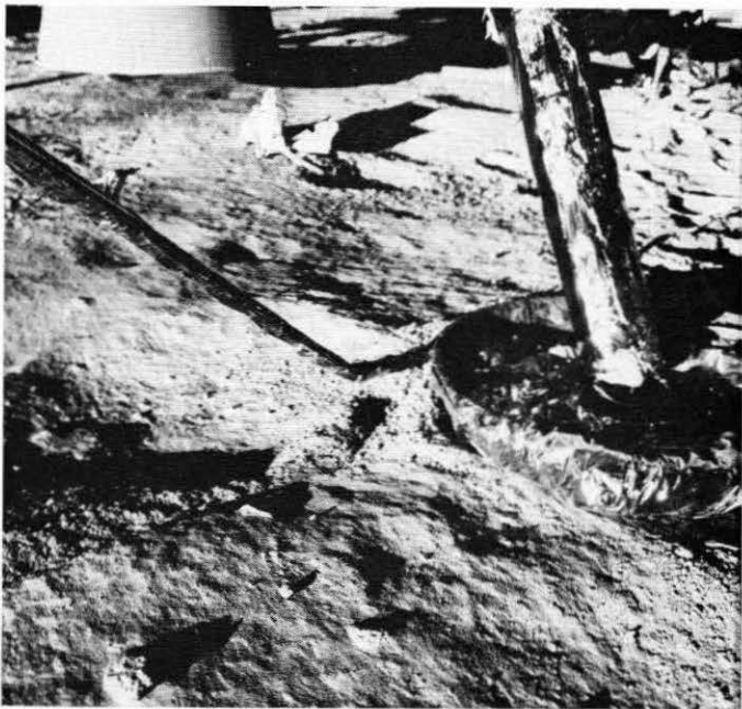
Fig. 3. Crater +y footpad and area under lunar module descent engine
