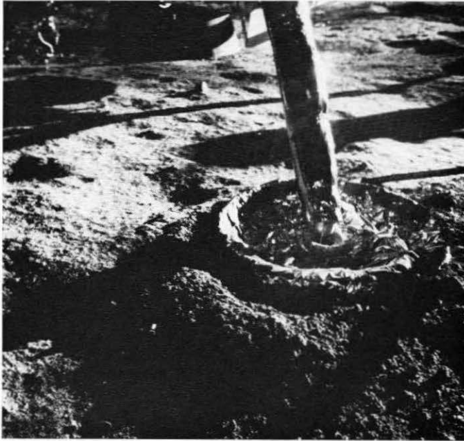
Fig. 2. Penetration of -y footpad; footpad diameter 37 in.
