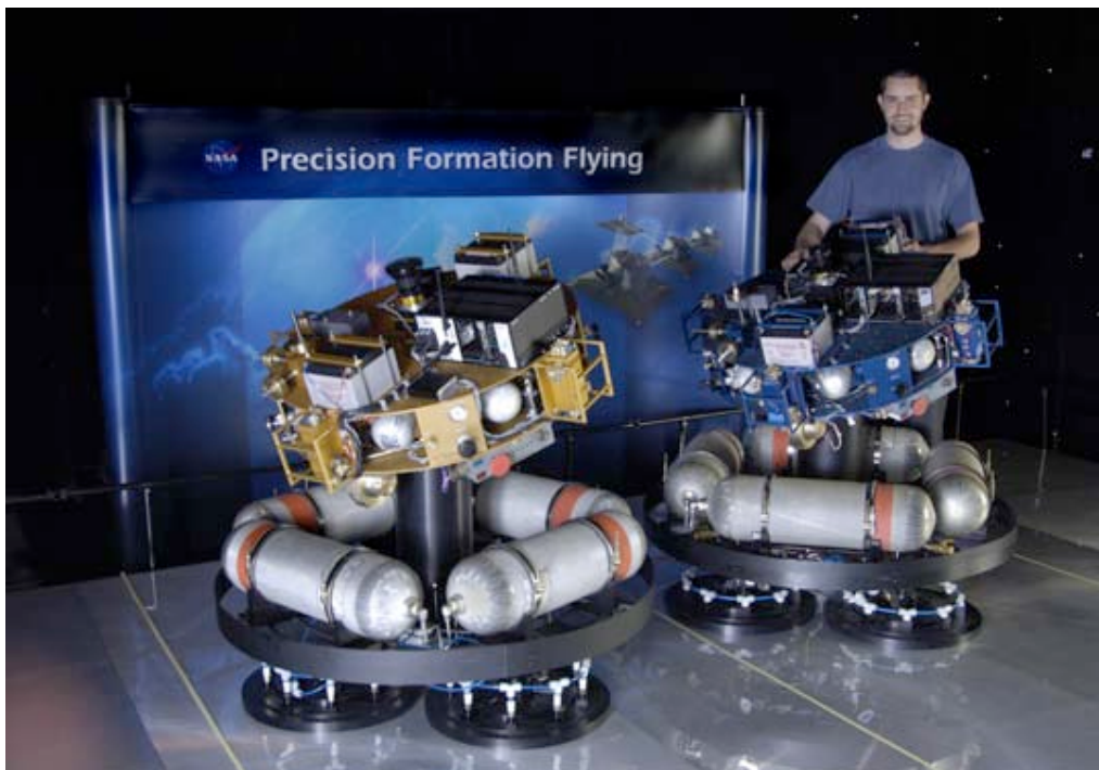
Figure 4-23. The Formation Control Testbed (FCT). Shown here are the two robots of the FCT. Each robot carries canisters of compressed air that allow them to float off a polished metal floor. The floor is flat to within 2 one-thousandths of an inch and spans a much larger area than shown here. The robots serve as the hardware interface and testing ground for flight software developed for space applications in formation flying. (Courtesy Caltech/JPL/NASA)
