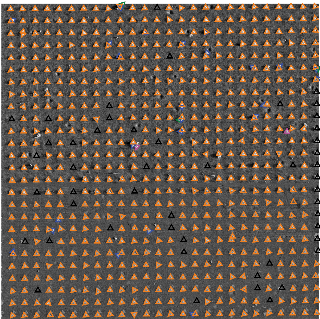
Figure S21. 35 mM Mg 2+ , annotated AFM. Other conditions are: 110 pM origami, 5 mM Tris, pH of 8.35, 60 min incubation, period of 400 nm. Triangular outlines provide a classification of an origami and/or binding site: empty binding site , first origami on a site , second origami on a site , third origami on a site , or origami bound to the background .
