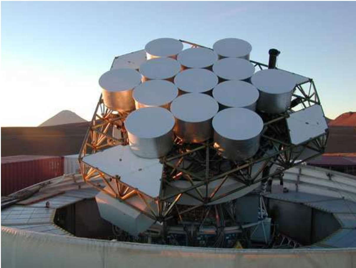
Figure 1: The Cosmic Background Imager. For the polarization observations, the 13 90-cm Cassegrain antennae were arranged in this hexagonal close-packed configuration on the rotating, alt-az mounted platform, with six adjusted to be sensitive to right-hand circularly polarized radiation and seven to left-hand circularly polarized radiation. By correlating the signals from the antennae in pairs, 78 interferometer baselines are obtained ranging in length from 1.0 to 3.5 m.
