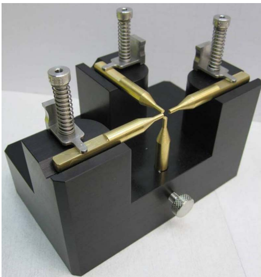
FIG. 7. Transfer block device used for transferring the sample to grind and polish any necessary face, while preserving the optical plane and bisectrix locations.
