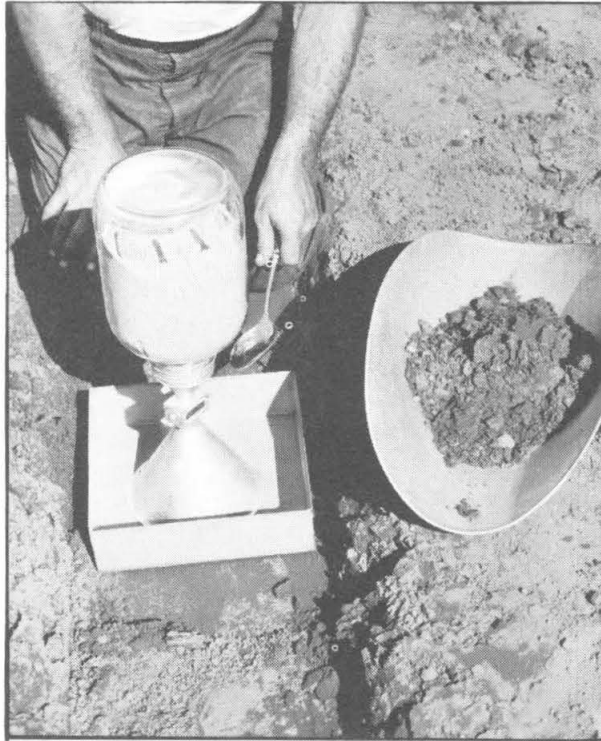
(A) Density Measurement of Sand-Replacement Method
