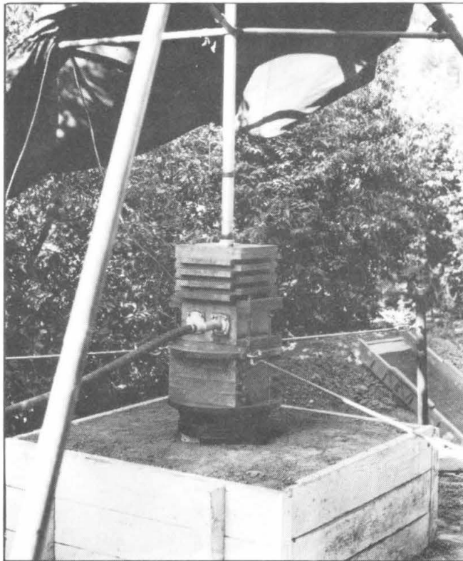
(A) Lazan Oscillator mounted on Skids for Tests L7-1
