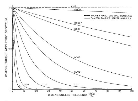
Fig. 4. Damped Fourier amplitude spectrum curves indicating the response  $|F_d|$  of an oscillator of natural frequency  $\omega_n$  and percentage of critical damping,  $\xi$ , to a delta function input at time t=0.
