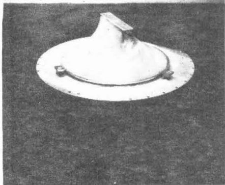
FIG. 2 RUBBER SHEET STRETCHED BETWEEN CIRCULAR SECTION AND RECTANGULAR SECTION AT DIFFERENT ELEVATIONS. HORIZONTAL SECTIONS OF THIS SHAPE WERE USED TO RELATE AREA TO CROSS-SECTION SHAPE FOR THE FINAL NOZZLE DESIGN.
