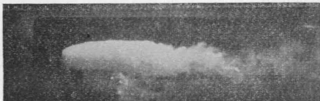
FIG. 8—CAVITATION ON A SQUARE END CYLINDER WITH AXIS PARALLEL TO FLOW. NOTE SLIGHT CAVITATION ON SUPPORT. (FLOW LEFT TO RIGHT.)
