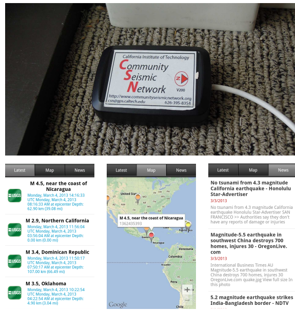
Figure 1: CSN volunteers contribute data from low-cost accelerometers (above) and from Android smartphones via a CSN app (below).
