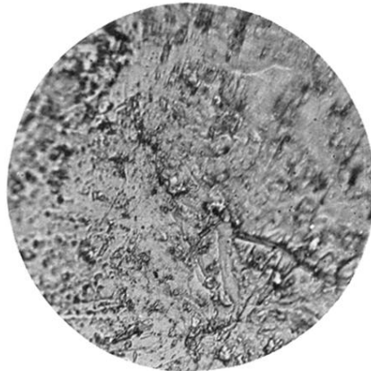
Fig 2. Microphotograph of the surface of a flake from which \text{SiO}_2 and Fe were removed (0001) plane, 495\times magnified. The surface is much more uniform and shows a pattern indicating the crystallographic symmetry.
