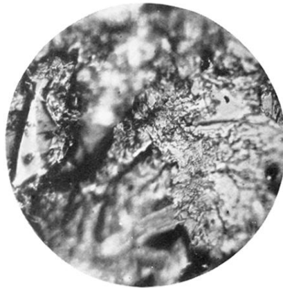
Fig. 1. Microphotograph of the surface of a flake of untreated Ceylon graphite, 495\times magnified. It shows the inhomogeneity due to adhering crystal fragments.
