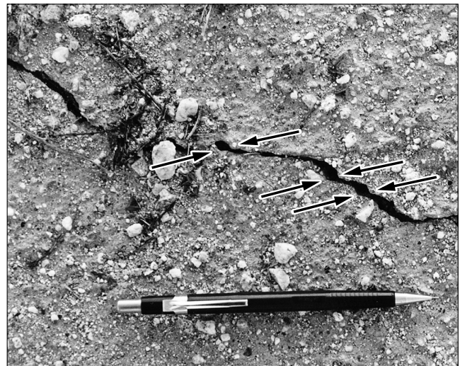
Figure 7. Photograph of fracture along San Andreas fault east of the main wash in Box Canyon with right-lateral component of slip. Fracture formed as aseismic slip in fall of 1997; pencil is oriented parallel with local trend of fault. Arrows point to matching breaks in soil crust; arrows are oriented parallel to slip azimuth. Photograph taken 22 November 1997.
