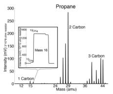
Figure 1: Full spectra of propane as measured on MAT253-Ultra [1] DeNiro, Epstein (1977) *Science* Volume 197, 261-263. [2] Eiler et. al (2012) this volume.
