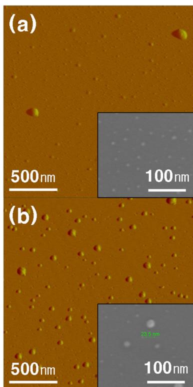
FIG. 1. (Color online) AFM image and SEM image of the evaporated nanometer sized Ni-dots on P-GaN surface with controlling its grain size of (a) 2-7 nm and (b) 20-50 nm, respectively, by evaporation time and temperature.
