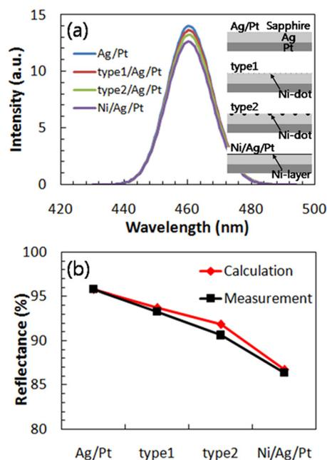
FIG. 4. (Color online) For each of the p-metal structure (inset of figure (a)), (a) calculated reflection spectra by 2-dimensional finite-difference time-domain method and (b) plots of measured and calculated reflectivity.
