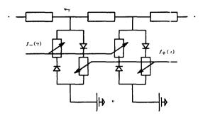
Figure 6: The structure of a diffusive network composed of ideal diodes and resistors, computing the top and bottom functions.
