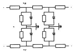
Figure 2: The structure of a diffusive network composed of ideal diodes and resistors, computing the top and bottom functions.
