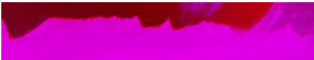
Figure 2-4. A colour composite from the North African coast comprised of R: AATSR nadir 0.55 \mu m, G: Null values, B: AATSR forward 0.55 \mu m. The apparent pink edges along the coast line are due to poor co-registration between the nadir and forward views. (Taken from AATSR orbit: 32768, 6 th June 2008)
