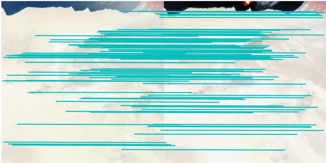
Figure 2-8. The first 100 matched tie-points between the forward and nadir AATSR views derived by SURF from the 0.55\mu\text{m} channels from the images presented in Figure 2-3. Incorrect matches are generally indicated by those tie-point pairings that do not conform to the general consensus (i.e. lines which are not parallel). It is evident from the above example that there no incorrect matches, i.e. all lines are parallel.
