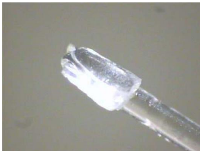
Figure 4.7 Example of a multilayered (SR)-naproxen crystal (size 0.6mm x 0.3mm x 0.07mm). This was the largest crystal grown in the attempts to obtain single crystals over a period of a few months.
