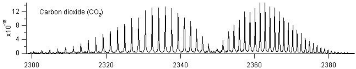
Figure 2.2: CO 2 absorption lines centred on the \nu_3 vibration mode ( \tilde{\nu} = 2349 \text{ cm}^{-1} ). Each line represents a transition in energy state, and the strength of the line (here expressed as \text{cm}^{-2}/\text{molecule} ) represents the probability of a transition to occur. Source: PNNL data from HITRAN website ( http://vp1.astro.washington.edu/spectra/co2.htm ).
