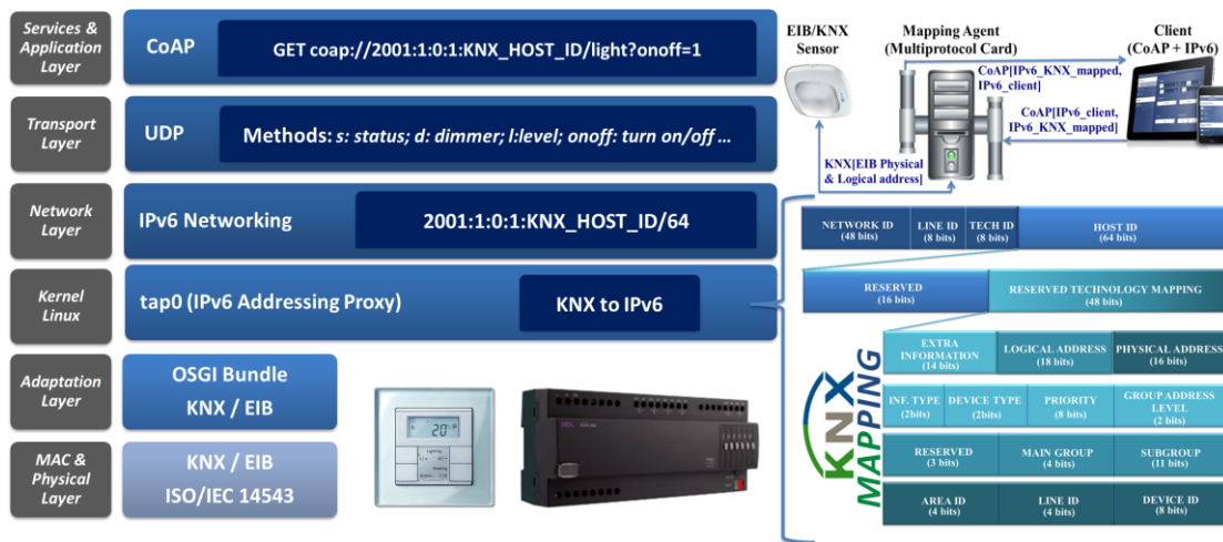
Figure 5. Left: Internet integration stack instance for KNX integration. Right: KNX mapping from native addressing to IPv6 and translation process.
