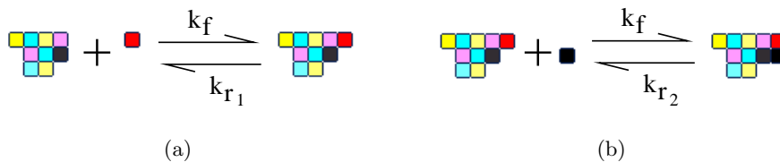
Fig. 5. Growth of tile assemblies based on (a) formation of a single bond, with energy \Delta G_1 and reverse rate k_{r_1} = e^{\Delta G_1/kT} , and (b) formation of two bonds simultaneously, with energy \Delta G_2 and reverse rate k_{r_2} = e^{\Delta G_2/kT} .
