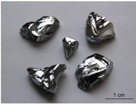
FIG. 1. (Color online) As-prepared \text{Ba}_8\text{Ga}_{16}\text{Ge}_{30} crystals grown in excess gallium.
