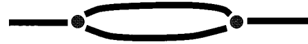
FIG. 4. Doubly linked nodes. A pair like this can interrupt an otherwise straight string or act as a kink.
