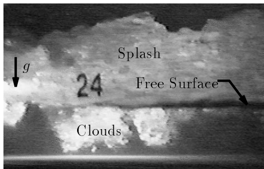
FIGURE 5: A photograph looking beneath the free surface at the periodic bubble clouds; \theta \approx 26^\circ , \phi \approx 15^\circ , and the flow is from right to left.
