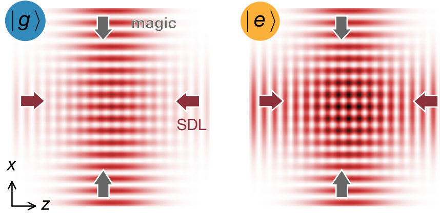
Figure 2.9 – Schematic of lattice potential experienced by ground-state (left) and excited-state atoms (right) in the presence of a 670 nm state-dependent lattice along z and a magic-wavelength lattice beam along x (dimensions not to scale). |e\rangle atoms experience a larger potential depth by a factor p = 3.3 than |g\rangle atoms along the SDL for the same light intensity while the perpendicular lattice confinement is identical for both species.
