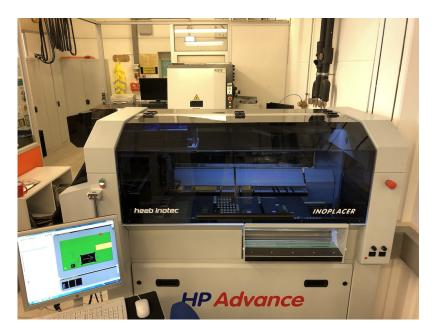
Figure 5.3: Fully automatic heeb inotec inoplacer HP Advance SMD loading machine.
