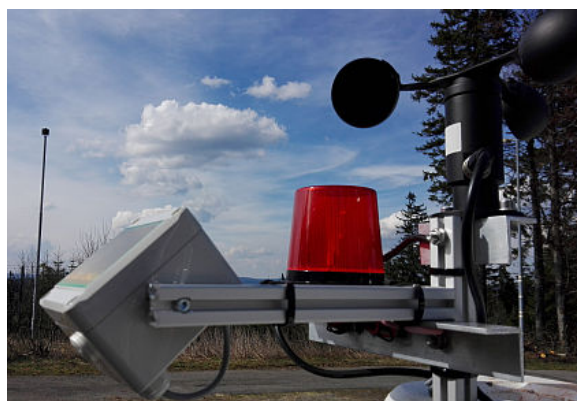
(b) CORAL's precipitation and wind sensors.
