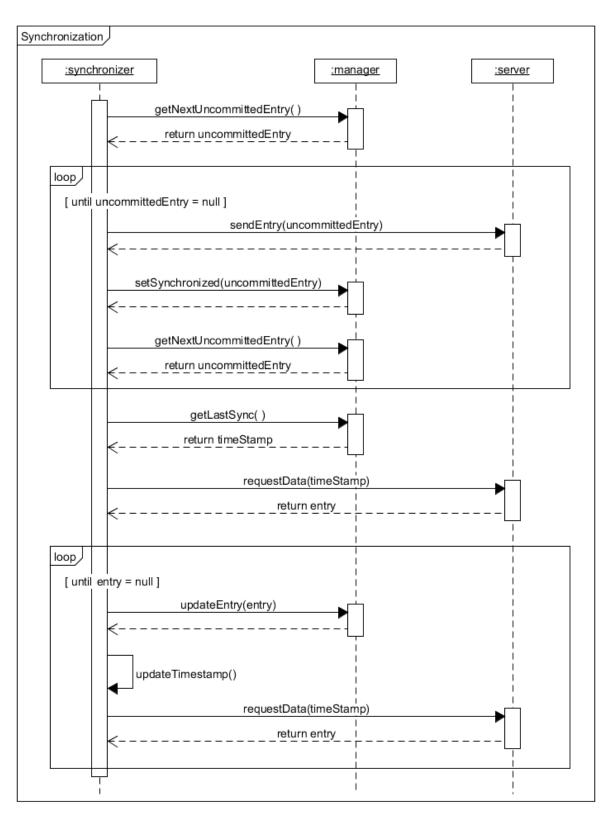
*Figure 3.7:* Simplified visualization of the synchronization, displaying the commit of changed entries to the server and new data from the server.
