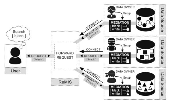
Figure 4.4: Sketch of the Reverse-Mediated Information System. The data owners can register their databases to the system on their own. The necessary mediation setup is executed by a wizard dialog. The architecture forwards the user request to the data sources where the request is mediated.
