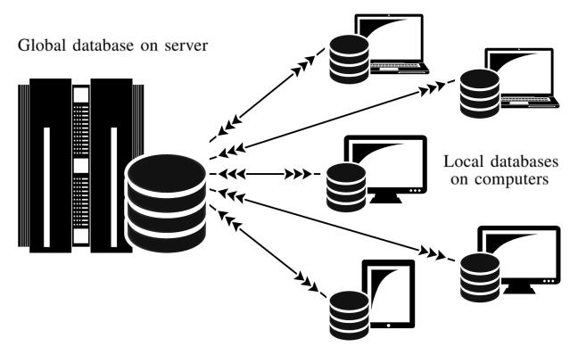
*Figure 3.2:* The local clients are connected to the global server. The synchronization allows data exchange, so data can be recorded on the local machines, but can be backed-up and shared via the server.
