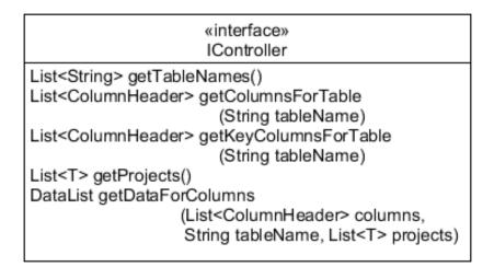
Figure 5.3: Schematic representation of the IController.
