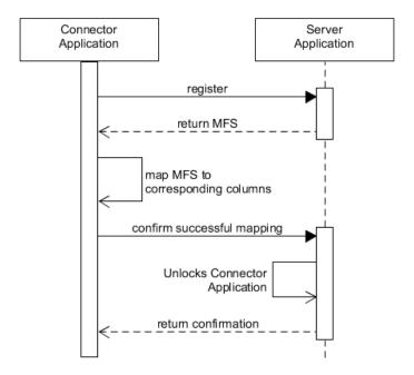
Figure 4.8: Sequence diagram of the registration process.
