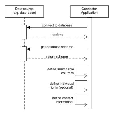
Figure 4.7: Sequence diagram of the initialization process.
