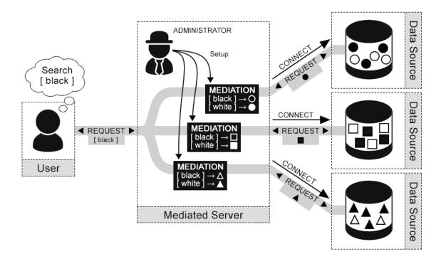
Figure 4.3: Sketch of the well-known Mediator-based architecture. A central administrator is required to connect the data sources and to mediate the requests from the user. The administrator has to know each data source to be able to connect them.
