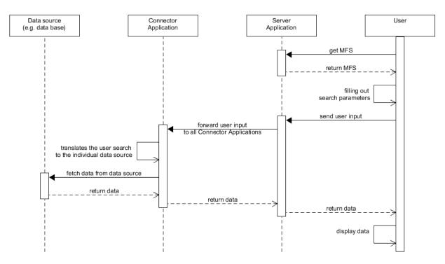
Figure 4.9: Sequence diagram of the process to fetch data from the single data sources.
