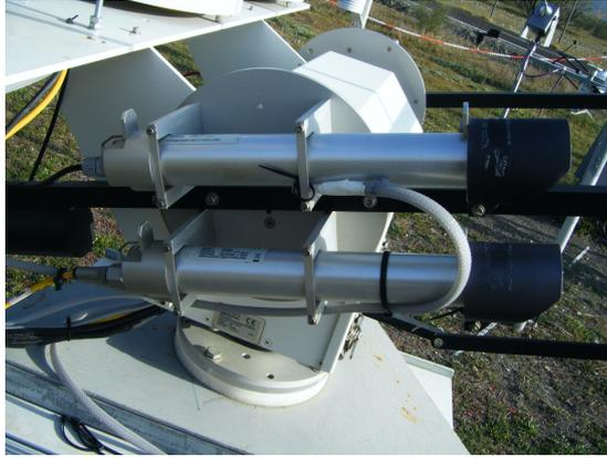
**Figure 3.8:** Pyrheliometer of the type Kipp & Zonen CHP1 at the PSA.
