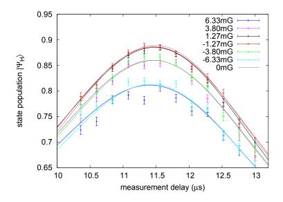
Figure 5.12.: Dependence of the rephasing on magnetic fields in the y-direction.
