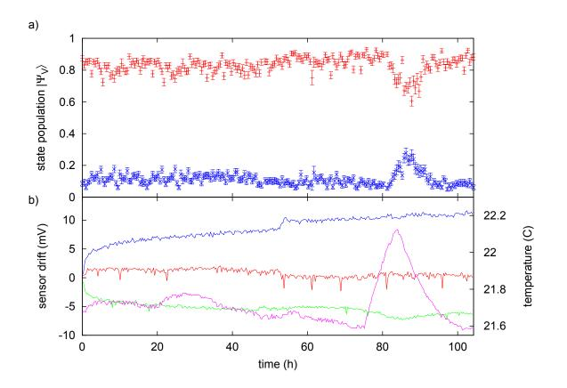
Figure 5.7.: a) Stability of the prepared atomic states  $|\Psi_H\rangle$  (blue) and  $|\Psi_V\rangle$  (red), measured at a time delay of 55  $\mu$ s over 104 hours. After 76 h the temperature stabilization of the air condition was switched off. b) Recorded voltage difference between the magnetic field sensors along the x- (red), y- (green), and z-direction (blue) during the calibration procedure. Additionally, the temperature (magenta) measured at the ion-getter pump is shown.
