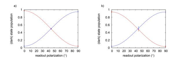
Figure 5.17.: Correlation measurement after optimal adjustment of all parameters before a Bell experiment (for photon polarizations |H⟩ = blue, |V⟩ = red). The number of settings is reduced to minimize the calibration time. a) Atom-photon correlations for the trap 1 setup. b) Atom-photon correlations for the trap 2 setup.
