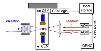
Figure 6.2.: Schematic of the state analysis in the Bell test. The output bit of the quantum random number generator (QRNG) selects which of the two AOMs is switched on. Each AOM provides a different polarization ( $\alpha$ ,  $\alpha'$ ) of the readout beam that determines the measurement direction. Detection events of the CEMs are recorded by a local storage (together with the random bit) to evaluate the result of each trial.
