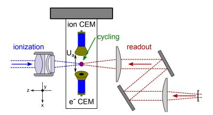
Figure 2.5.: Schematic of the setup with the respective laser beams of the state analysis. The readout and ionization beams are applied from opposite directions along the z-axis. The cycling beam is applied from the top. Channel-electron-multipliers (CEM) are placed inside the vacuum cell to detect the electron and the ion after an ionization event. The acceleration voltage between the two CEMs is  $U_a \approx 3.6 \,\mathrm{kV}...4.6 \,\mathrm{kV}$ .
