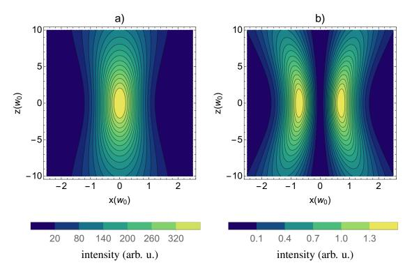
Figure 5.8.: Intensity profile in the focal region of the ODT beam (for y = 0). a) Transversal component  $|E_x|^2$ . b) Longitudinal component  $|E_z|^2$ .
