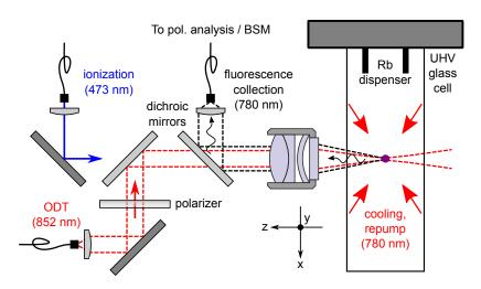
Figure 2.2.: Setup of the confocal microscope used to focus the dipole trap beam and the ionization beam to the atom and to collect fluorescence of the trapped atom. The fluorescence is coupled into an optical single-mode fiber that leads to a polarization analysis or a Bell-state measurement (BSM) apparatus. The shown layout corresponds to the trap 1 setup. Another atom trap (trap 2) used for this work has a different order of dichroic mirrors.
