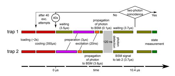
Figure 4.3.: Experimental sequence to entangle two Rubidium atoms. When atoms are loaded in both dipole traps, they are repeatedly prepared and excited to generate atom-photon entanglement. After 40 repetitions of the preparation-excitation cycle recooling of the atoms is necessary. When a two-photon coincidence is registered at the BSM detectors (within a certain photon detection time window) the setup switches to the state analysis.
