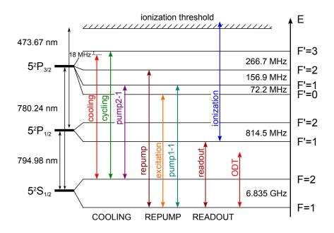
Figure B.1.: Laser frequencies and their labeling as used in the experiment.
