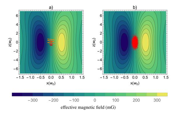
Figure 5.10.: Randomly calculated atomic trajectories (a) and positions (b) according to a thermal distribution, projected on the x-z-plane. The penetration depth into regions with an effective magnetic field  $B_{long}(\vec{x})$  is shown. The sign of  $B_{long}(\vec{x})$  changes at x = 0.
