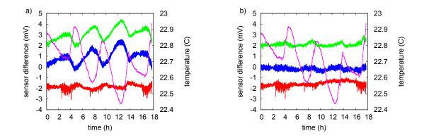
Figure 5.6.: Temperature correction for the sensor recalibration. Shown are the differences between the sensor voltages  $\Delta U$  (for the directions x (red), y (green) and z (blue)) for fluctuating temperatures of the magnet of the ion getter pump. The temperature varies (magenta) by about 0.5 K. a) Sensor differences according to equation 5.5 show fluctuations depending on the temperature. b) Fluctuations can be suppressed with additional temperature correction (equation 5.6).
