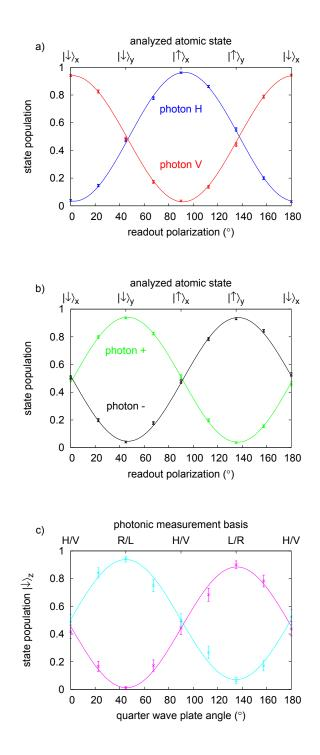
Figure 3.3.: Atom-photon correlations. In a) and b) the linear polarization of the readout laser is rotated, hence the atomic measurement basis is rotated by  $2\pi$  in the spin space. The basis of the photons is H/V in a) and +/- in b). In c) the atomic states are projected onto  $|\downarrow\rangle_z$  and the photonic basis is rotated.
