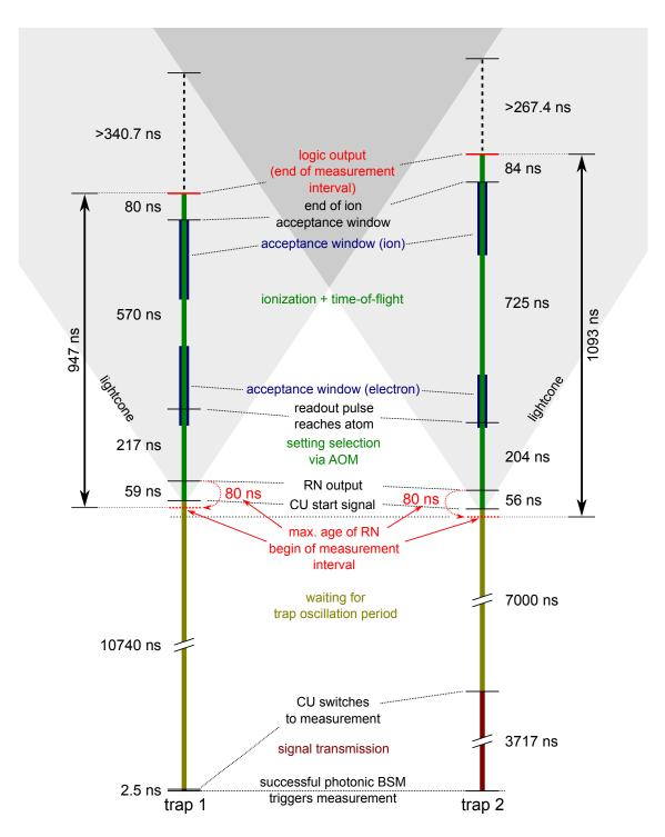
Figure 6.4.: Space-time diagram of the state measurements in trap 1 and trap 2.
