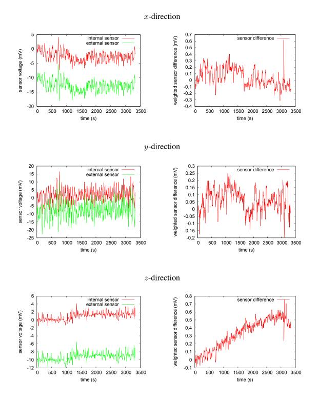
Figure 5.5.: Left: Output voltages of the internal and external (scaled with a factor of 0.1) sensor along three directions (set to 0 and -10 at t = 0). Fluctuations of more than 0.5 mVare associated with a change of the magnetic field. Right: The difference between the sensor voltages weighted with sensitivities  $s_i^{(i)}$  and  $s_e^{(i)}$  shows only small fluctuations (set to 0 at t = 0).
