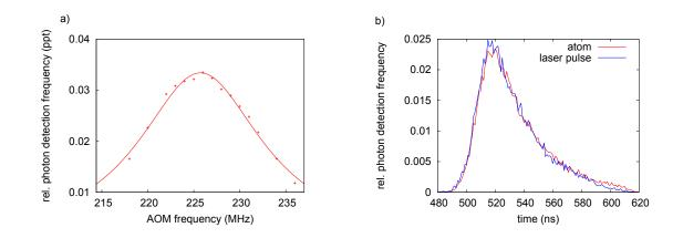
Figure 3.5.: a) Adjustment of the central frequency of the laser pulse to the frequency of the atomic transition  $5^2S_{1/2}$ ,  $F = 1 \rightarrow 5^2P_{3/2}$ , F' = 0. The laser frequency is varied with an AOM and the relative photon detection frequency at the APDs is measured. The data is fitted by a Lorentzian to determine the maximum. b) Measured arrival time histograms of photons originating from the atom (red) and laser pulse (blue) at the APDs. The calculated overlap is 0.994.
