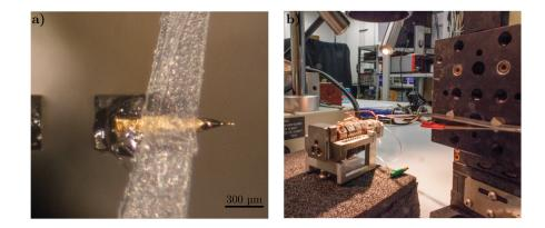
Figure A.15: Gluing a tip: a) View through the microscope on the glued tip. The tip is positioned on the upper prong of the tuning fork and fixed with a drop of epoxy glue. b) Setup for gluing a tip. The AFM stack is laid down with the tuning fork pointing up. The cut tip is hold by a pair of tweezers, fixed on the lower part of the micrometer stage.
