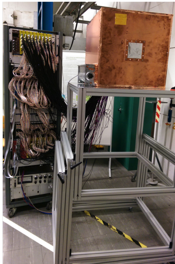
Figure 3.2.22: Photograph of the complete Compton camera setup, mounted on its support stand and together with the signal processing electronics. The Compton camera system is housed inside a (light-tight) Faraday cage, which includes a ventilation fan used to exchange the hot air from inside the box, as well as an entrance window. The entrance window is covered by a thin aluminum foil ( 30 \mu\text{m} ) in order to minimize the scattering probability for incoming photons. A backside slit was used as a feedthrough for the signal processing electronics cables of both the scatterer and absorber, directed to the signal processing and DAQ system standing in the back. The Compton camera box was placed on top of an adjustable stand, which offers an adjustable height range of 1 to 2 m.
