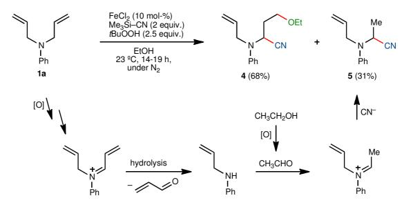
Scheme 3.5. Oxidative Cyanation of *N*,*N*-Diallylaniline in Ethanol (yields refer to isolated products after separation and purification by column chromatography).
