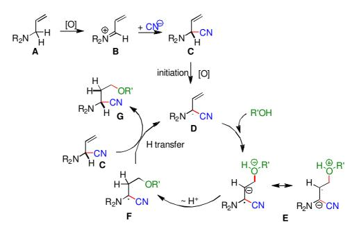
Scheme 0.6: Suggested mechanism for the oxidative C1-cyanation of the *N*-allyl group with subsequent anti-Markovnikov hydroalkoxylation.
