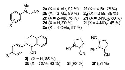
**Scheme 2.3.**  $\alpha$ -Amino nitriles obtained by FeCl<sub>2</sub>-catalyzed cyanations of aniline derivatives with trimethylsilyl cyanide and *tert*-butyl hydroperoxide.<sup>[34]</sup>
