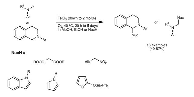
Scheme 1.11: FeCl<sub>3</sub> catalyzed oxidative coupling of tertiary amines with various nucleophiles.<sup>[23]</sup>
