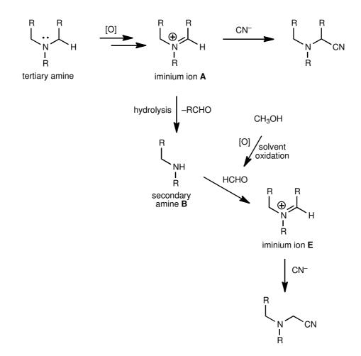
Scheme 0.2: Oxidative dealkylation of tertiary amines by FeCl<sub>2</sub> as the catalyst and *tert*-butyl hydroperoxide as the oxidant and subsequent trapping of the secondary amine intermediates.
