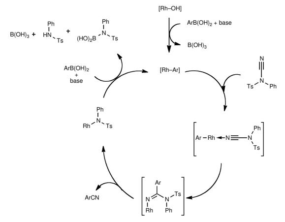
Scheme 1.22: Suggested mechanism for the Rh-catalyzed cyanation of boronic acids.<sup>[44a]</sup>
