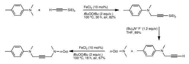
Scheme 1.7: Subsequent FeCl<sub>2</sub>-catalyzed oxidative couplings with two different tertiary amines.<sup>[20]</sup>
