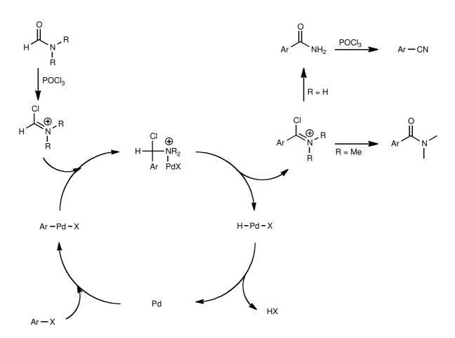
Scheme 1.30: Postulated mechanism for a Pd-catalyzed cyanation of aryl halides.<sup>[56]</sup>
