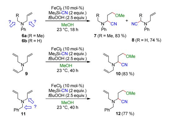
Scheme 3.6. Oxidative Cyanation/Hydroalkoxylation of the Monoallylamines **6a,b**, Triallylamine (**9**) and *N*,*N*-Diallylbenzylamine (**11**) (All reactions under dry  $N_2$  atmosphere. Yields refer to isolated products after chromatographic purification)
