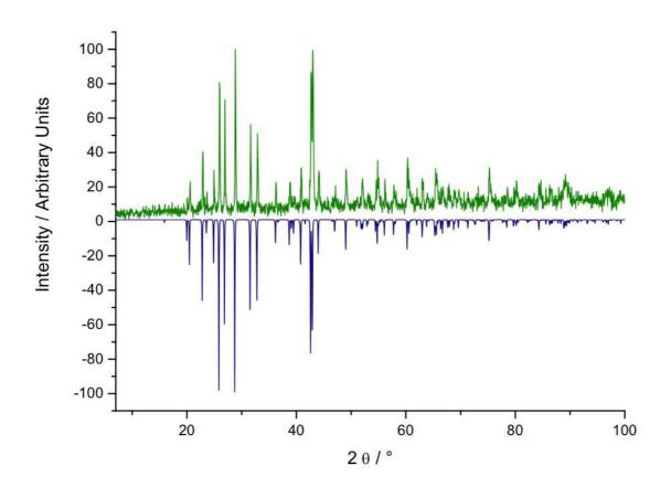
**Figure 4.1**. Reflections of the precipitated solid (upper line in green) agree with those that were previously determined for barite (BaSO<sub>4</sub>, lower line in blue, data from ref.<sup>27</sup>).
