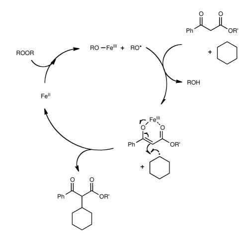
Scheme 1.6: Mechanism for the Fe-catalyzed alkylation of 1,3-dicarbonyl compounds as suggested by Li et al.<sup>[19]</sup>
