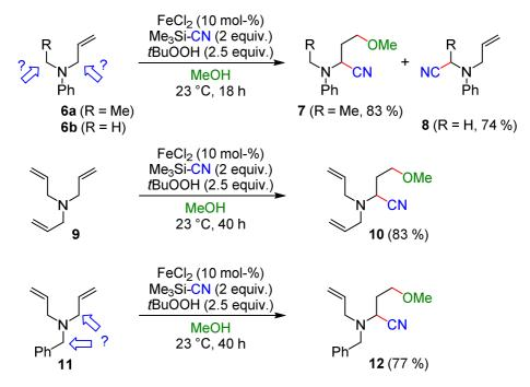
Scheme 0.5. Oxidative cyanation/hydroalkoxylation of the mono-allylamines, triallylamine and *N*,*N*-diallylbenzylamine.
