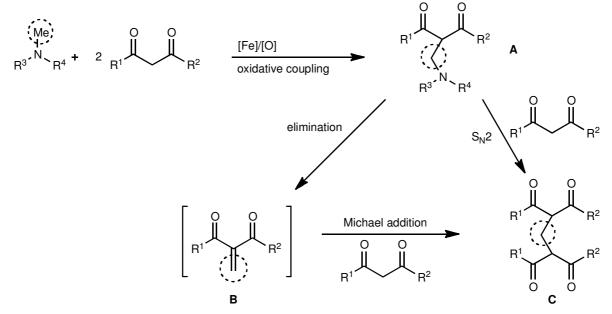
Scheme 1.10: Mechanistic study and suggested pathways for the iron-catalyzed CDC of *N*-methyl amines with 1,3-dicarbonyl compounds.<sup>[22a]</sup>
