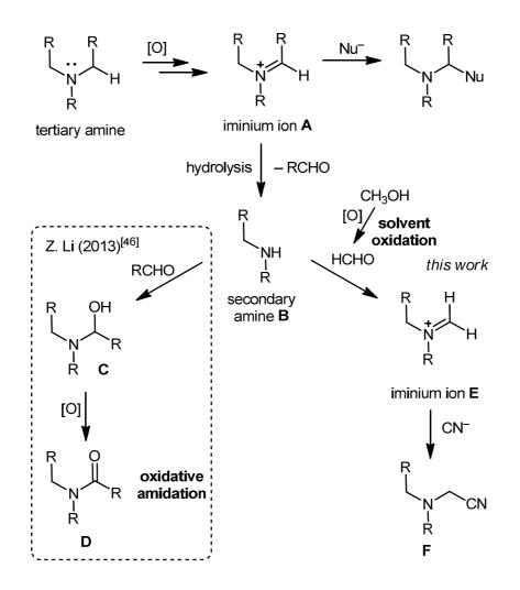
**Scheme 2.4.** Oxidative dealkylation of tertiary amines by FeCl<sub>2</sub> as the catalyst and *tert*-butyl hydroperoxide as the oxidant and subsequent electrophilic trapping of the secondary amine intermediates.
