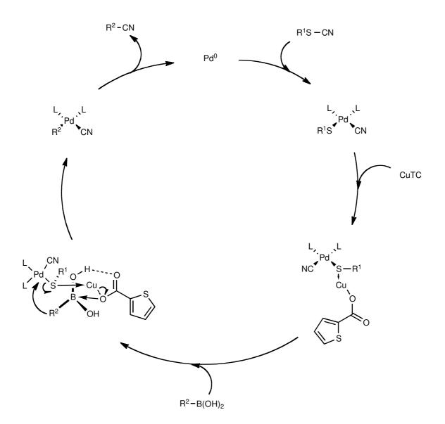
Scheme 1.33: Proposed mechanism, for the reaction of aryl- and alkenylboronic acids with benzyl thiocyanate.<sup>[61]</sup>
