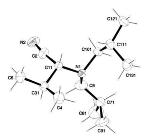
**Figure 2.1.** X-ray structure of **40** [as the molecules crystallized disordered a split model was applied (sof ratio 0.72/0.28), the Figure shows the main component only, thermal ellipsoids are drawn at the 50% probability level].<sup>[42]</sup>
