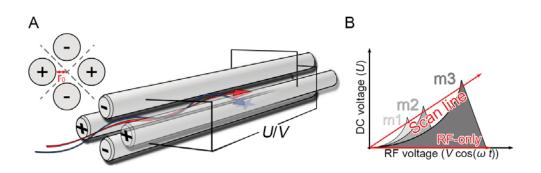
**FIGURE 5 | Schematic function of a quadrupole for mass selection or ion guiding. A** Conceptual construction of a quadrupole. **B** Diagram of quadrupole scanning and stabilization of ions (adapted from Barner-Kowollik et al., 2012 [58]).
