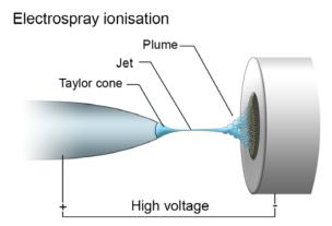
**FIGURE 4** | A schematic view of electrospray ionization (ESI). The flow rate of the liquid defines how well the Taylor cone and the desolvation of the electrospray plume perform (adapted from Hahne et al., 2013 [55]).
