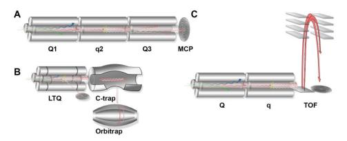
**FIGURE 8** | Components of QqQ, LTQ-Orbitrap, and Qq-TOF instruments. A Arrangement of quadrupoles of a QqQ instrument, with mass selection quadrupoles (Q1 and Q3), and a fragmentation cell (q2). B Dual analyzer arrangement of LTQ-Orbitrap hybrid instruments. C Working principle of Qq-TOF instruments with a mass selection (Q), a collision cell (q), and a TOF analyzer.
