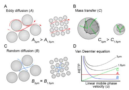
**FIGURE 3** | Influence of physical phenomena on chromatographic resolution. A-C: Schematic depiction of factors influenced by particle size. D: The effect of flow rate on chromatographic plate height according to the van Deemter equation (adapted from Meyer, 2013 [49]).
