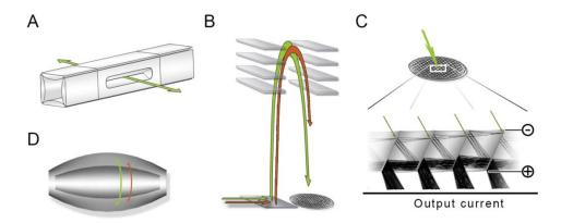
**FIGURE 7 | Mass analyzers and detectors used in modern mass spectrometers. A** Linear ion-trap quadrupole with scanning capability. **B** Orthogonal time-of-flight (TOF) system with a reflector. **C** Working principle of multi-channel plate (MCP) electron multiplier detector. **D** Schematic of an Orbitrap mass analyzer depicting the central and outer electrodes. (Adapted from Gross and Roepstorff, 2011 [56]).
