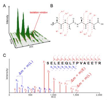
**FIGURE 6 | Peptide mass selection and fragmentation. A** 3D elution peak of peptide isotopepatterns. **B** Ion series annotation generated during peptide backbone fragmentation. **C** Fragmentation spectrum and peptide sequencing principle. (Adapted from Steen and Mann, 2004 [61]).
