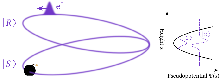
Figure 11: Sketch of a modified IFM scheme, similar to the one proposed by Putnam and Yanik (2009) shown in Fig. 9. The difference in the modified scheme is that the two paths of the electron corresponding to the states |R\rangle and |S\rangle are not parallel. For most of the paths, their distance is large enough that tunneling does not occur. The paths only intersect in a small region where they either come close enough for tunneling or may even merge to a single well (as shown in the pseudopotential plot on the right), allowing an exchange of amplitude between them.
