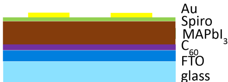
Figure 6-6: Standard solar cell layout, where the perovskite light absorber is sandwiched between a spiro hole conductor layer and a C_{60} electron selective contact.
