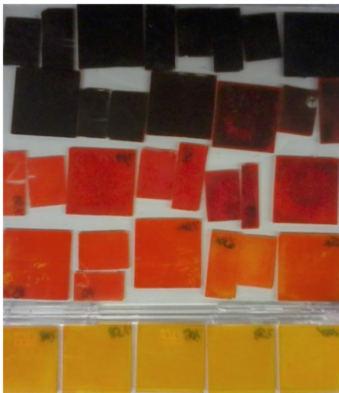
Figure 2-12: Photograph of a series of \text{MAPbI}_{3-x}\text{Br}_x perovskites ranging from 100 % iodide content (top left) to 100 % bromide (bottom right). The change in band-gap energy can be observed as color change.
