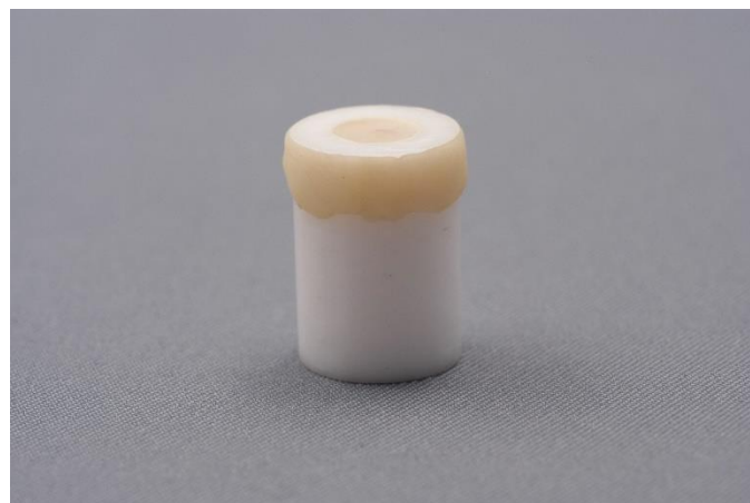
Figure 42 The Teflon cylinder serving as a cavity model. Flowable composite was applied to the outer contour simulating enamel in order to serve as a reference point for the rigid registration.
