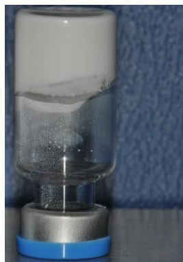
Figure 33: Flow behavior of a suspension with 300 mg/mL micronized API when vial is turned upside down.
