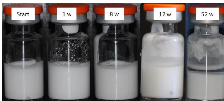
Figure 29: Sedimentation behavior of suspension with 300 mg/mL API at different time points.
