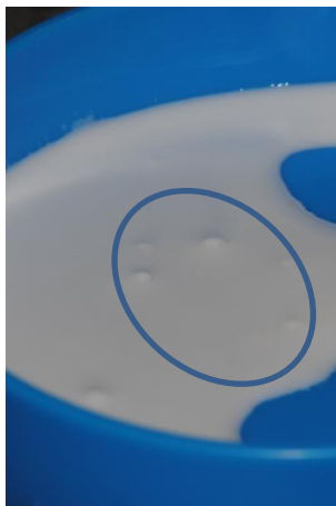
Figure 84: Agglomerates observed for the formulation containing 2 mg/mL DMPG and 150 mM NaCl after 4 weeks storage.
