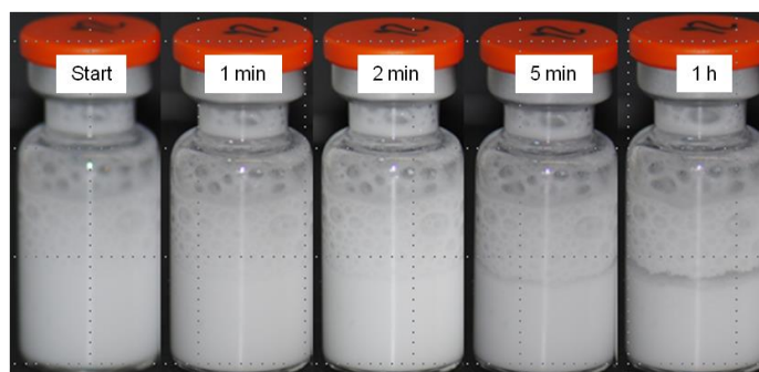
Figure 28: Sedimentation behavior of suspensions with 100 mg/mL API at different time points.
