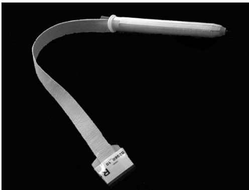
Fig.1: Writing stylus with force sensor matrix wrapped around the surface
