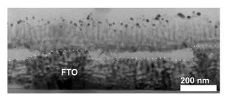
**Figure 4.7:** Damaged FTO is found as an indication for the harmfullness of a long anodization step.
