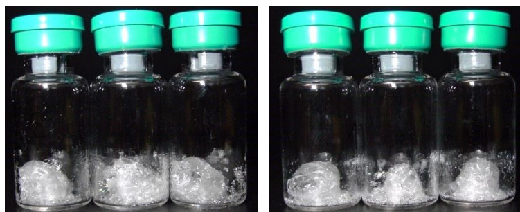
Figure 5.1: Macroscopic appearance of products aggressively freeze-dried samples from 5% (wt/wt) sugar solutions (process settings: p_c=1 mbar, T_s=45 °C). Left picture shows sucrose based samples, right picture trehalose based.
