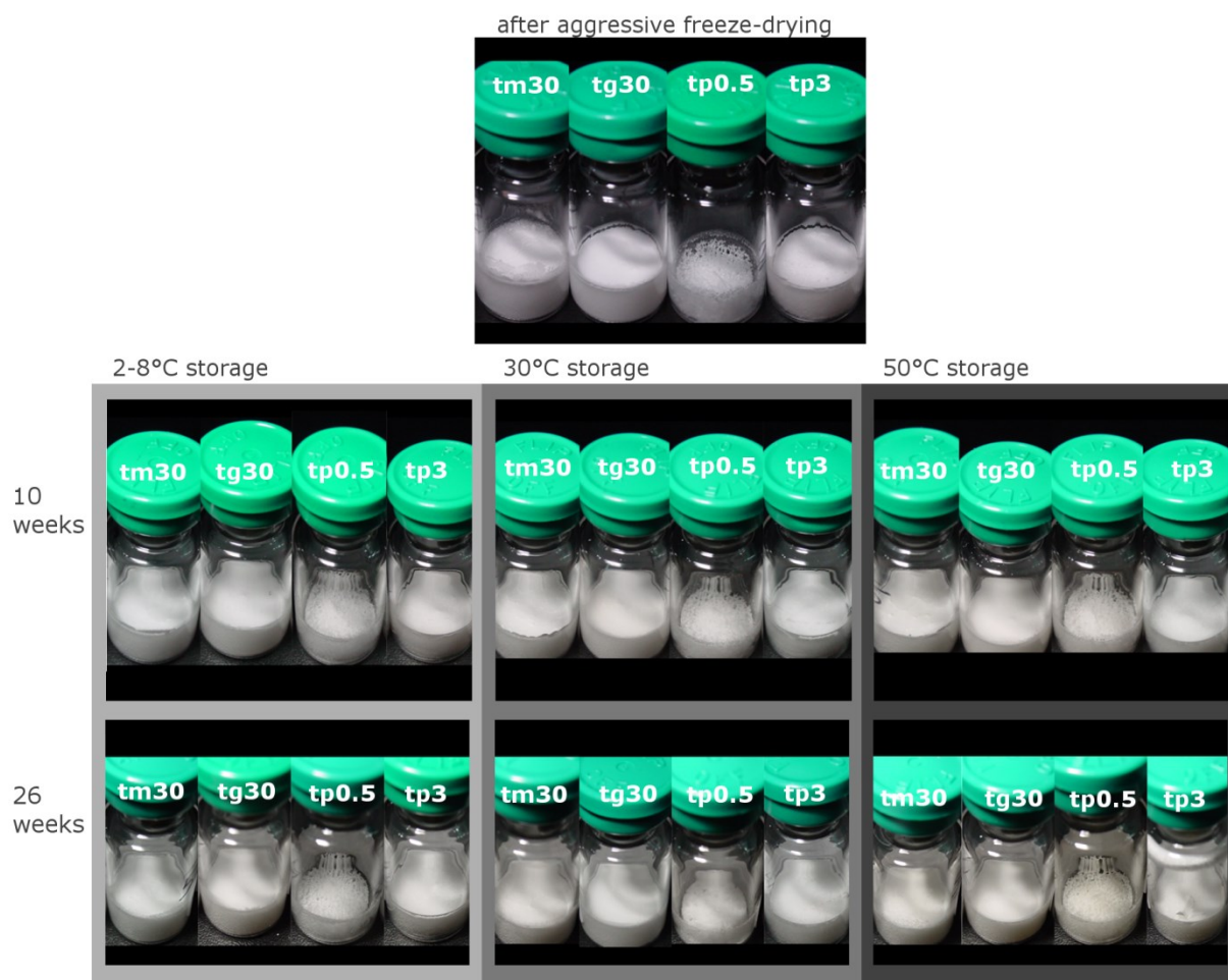
Figure 6.20: Macroscopic appearance after storage of aggressively freeze-dried samples at 2-8 °C, 30 °C, and 50 °C for up to 26 weeks (trehalose-based formulations contain bulking agents and 1 mg/ml mab_T1; tm30 \triangleq tre:man 10:30, tg30 \triangleq tre:gly 10:30, tp0.5 \triangleq tre:phe 10:0.5, tp30 \triangleq tre:phe 10:3).
