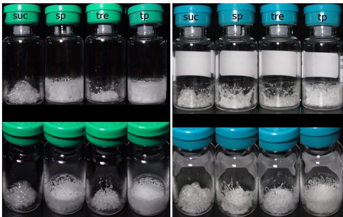
Figure 5.22: Macroscopic appearance of lyophilizates aggressively freeze-dried from sugar based formulations containing 1 mg/ml (left picture) or 10 mg/ml (right picture) mab_T1 (suc: sucrose; sp: sucrose:phenylalanine 10:0.5; tre: trehalose; tp: trehalose:phenylalanine 10:0.5).
