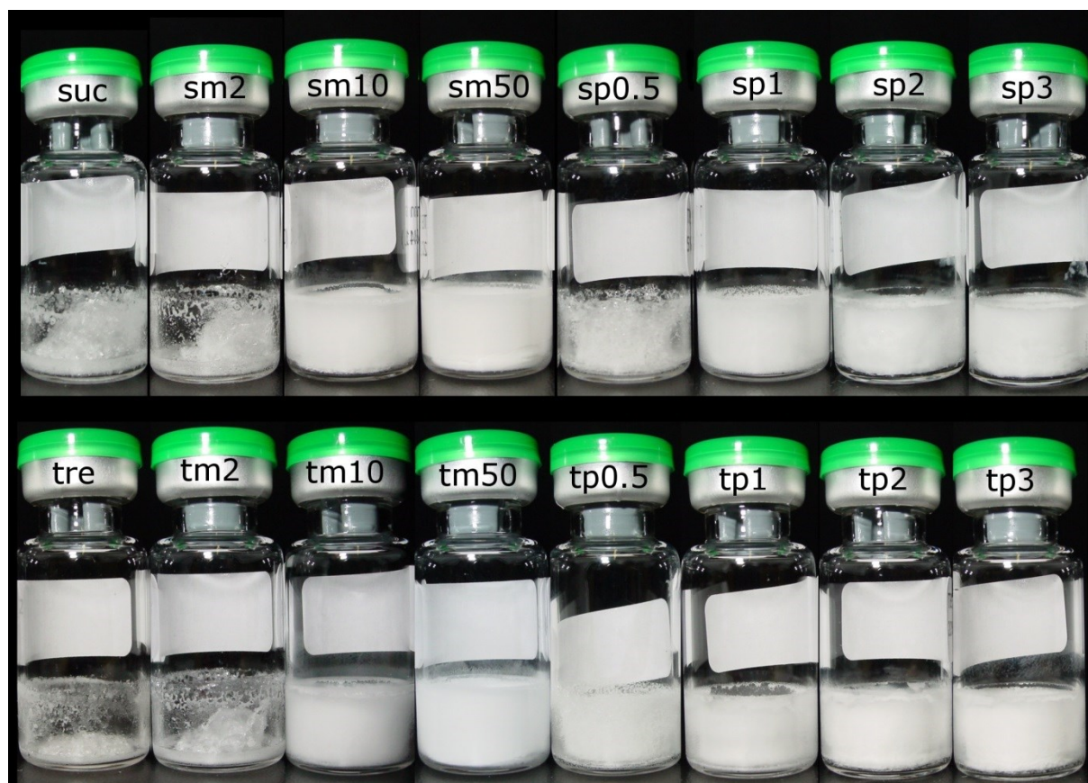
Figure 5.6: Macroscopic appearance of aggressively freeze-dried formulations containing different amounts of bulking agents (mannitol or phenylalanine), showing an overall comparable appearance between sucrose and trehalose (see text for sample description; process settings: p_c=1 mbar, T_s=45 °C).
