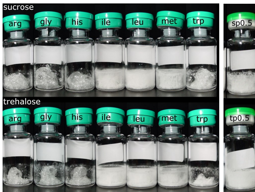
Figure 6.25: Macroscopic appearance of aggressively freeze-dried sugar-based formulations containing different amino acids at a sugar to amino acid ratio of 10:0.5 (upper row sucrose based, lower row trehalose based). For comparison suc:phe 10:0.5 (sp5) and tre:phe 10:0.5 (tp0.5) is shown.
