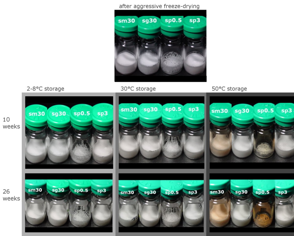
Figure 6.21: Macroscopic appearance after storage of aggressively freeze-dried samples at 2-8 °C, 30 °C, and 50 °C for up to 26 weeks (sucrose-based formulations contain bulking agents and 1 mg/ml mab_T1; sm30 \triangleq suc:man 10:30, sg30 \triangleq suc:gly 10:30, sp0.5 \triangleq suc:phe 10:0.5, sp30 \triangleq suc:phe 10:3).
