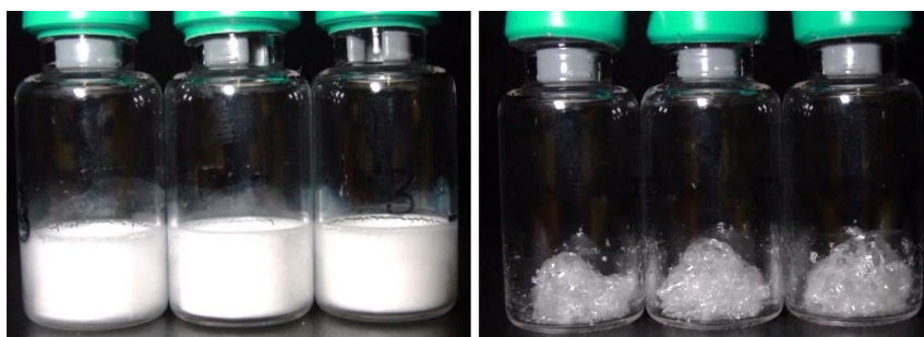
Figure 1.7: Macroscopic appearance of non-collapsed (left) as well as collapsed (right) lyophilizate (freeze-dried from 5% wt/wt aqueous sucrose solution)
